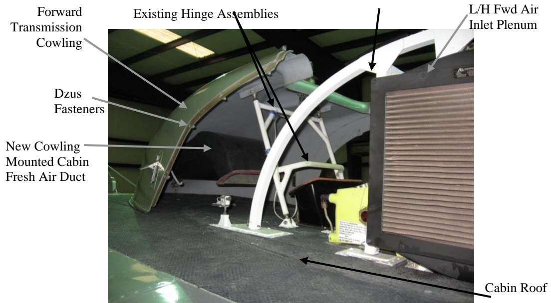
Figure 3-21 Forward Transmission Cowling on Roof
